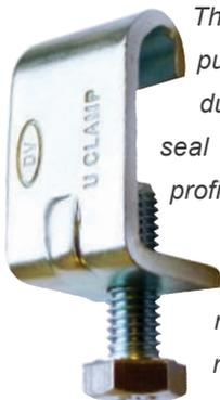
The New nose design ensures joint is pulled together horizontally and parallel to duct internal surface - maximising the air seal and minimising the tendency for the profiles to tilt and open up internally within the duct when the clamps are tightened. This in turn lowers the system energy running costs - due to better joint seal rather than using snap or drive clips.
