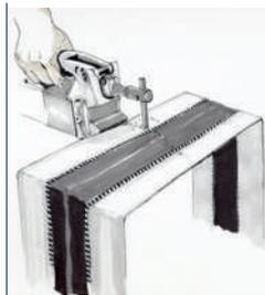
Spot-weld the steel and form to the desired shape.
