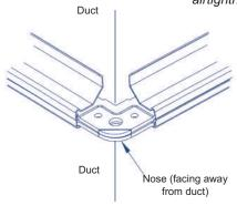
airtightness of the completed joint. If any burring has occurred during the cutting of the flange, this must be removed before assembly.
