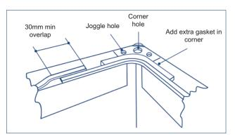
Assemble the ductwork by the use of nuts and set screws fitted into the corner holes. If necessary align the corner holes by use of the joggle holes. The nuts and screws should be finger tight at this point.
