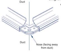
Fully insert four corners into the flange to form a rectangle frame as shown. Care must be taken to ensure the legs of the corners are fully inserted into the flange, the 'nose' on the corner faces away from the duct on which the frame is to be fitted.
