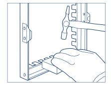
Complete the fit by mounting the remaining door into the frame and tighten the camlocks to the degree of tightness required - do not over tighten. Make sure also that the retaining wire is not snagged between the door and frame.
