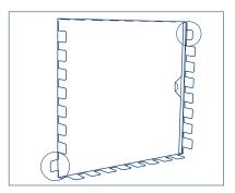
Using a support to hammer against, tap over the remaining metal tabs on the fitted subframe and ensure that all tabs are knocked over and the sealing gasket is under compression on all faces, including the corners.
