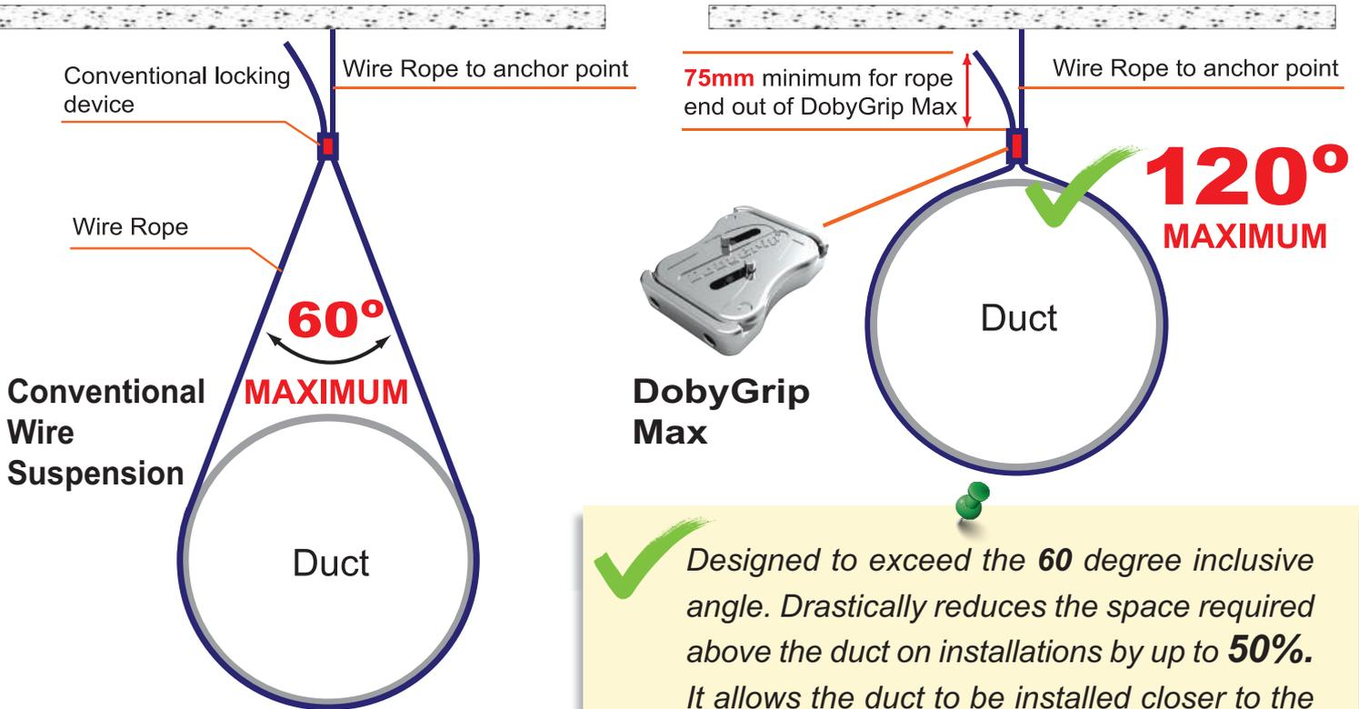
✓ Designed to exceed the 60 degree inclusive angle. Drastically reduces the space required above the duct on installations by up to 50%. It allows the duct to be installed closer to the suspension point and reduces the length of wire rope required.
