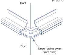
airtightness of the completed joint. If any burring has occurred during the cutting of the flange, this must be removed before assembly.
