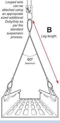
Allows for inspection access into services and further adjustment if required. For use with static loads only. 60° Max angle.
